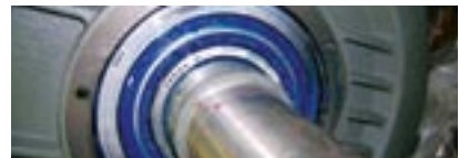
Oversized NSK/SKF bearings with Polyrex EM grease
